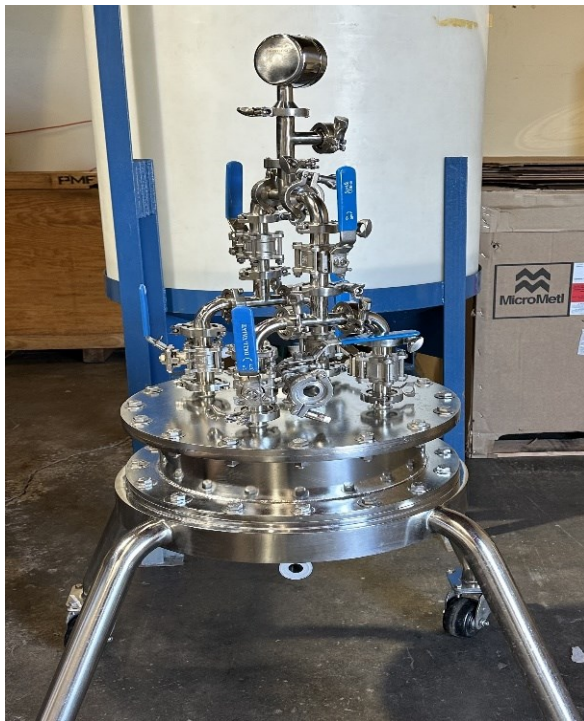
10L Superflo® Column packed manually with Sepaflo® Q resin
