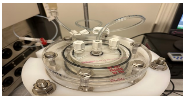
50ml Column packed with Q Sepharose and hetp run on the QuantaSep Trusty 100 with an asymmetry factor of 1
